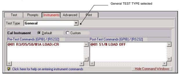
(i) **Note**: The PSU voltage should be set to 5 Volts to avoid excessive dissipation in the PSU adapter You can send a command to turn off the load after the test. (*Post Test Commands*)
